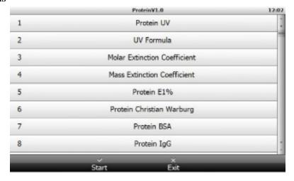
TL6 equipped with a variety of build-in protein quantitative detection methods, including Bradford, BCA, Lowry, Biuret, A280 method (Christian Warburg, BSA, IgG, Lysozyme, molar extinction coefficient, mass extinction coefficient, E1%), UV method and UV formula method etc.. TL6 supports up to 27 standard samples (including repeated measurement samples) for building standard curve. The standard curve can be directly displayed on the LCD screen, printed or saved to method.
